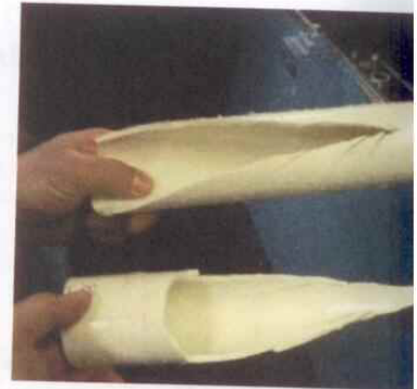
FIGURE 723.1B PLASTIC SHARD FROM COMPRESSED AIR
