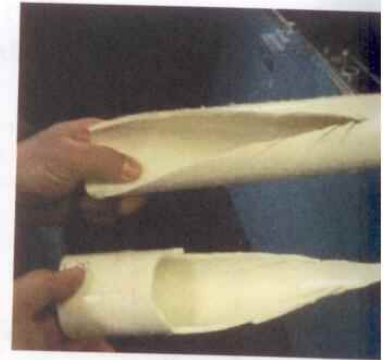
FIGURE 723.1B PLASTIC SHARD FROM COMPRESSED AIR
