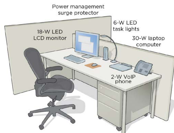
Figure 5. Diagram of an example low-energy workstation. Illustration by Matthew Luckwiltz, NREL
