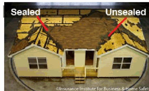
Figure 9 - Photograph of the front of the duplex after shingle and underlayment removal using high winds, illustrating the sealed roof deck (on the left) and the un-sealed roof deck (on the right).
