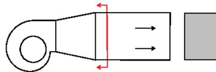
Fan outlet area for a fan tested with an outlet diffuser is the cross-sectional area at the diffuser outlet, which is also equal to the test duct cross-sectional area.
