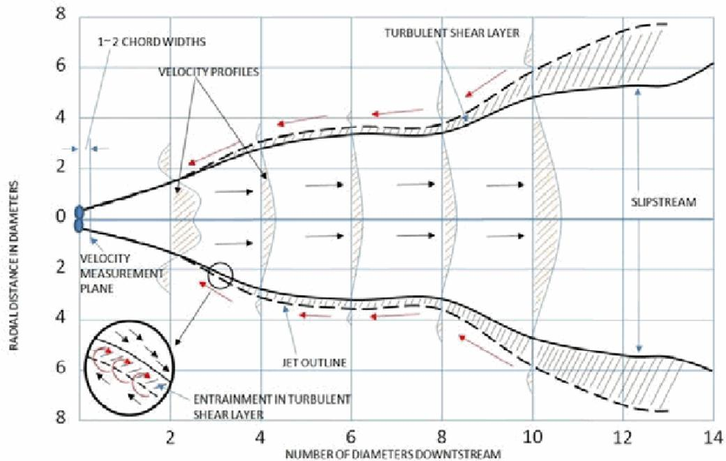
NOTE: TEST ROOM NOT LESS THAN 30 DIAMETERS LONG X 20 DIAMETERS WIDE
