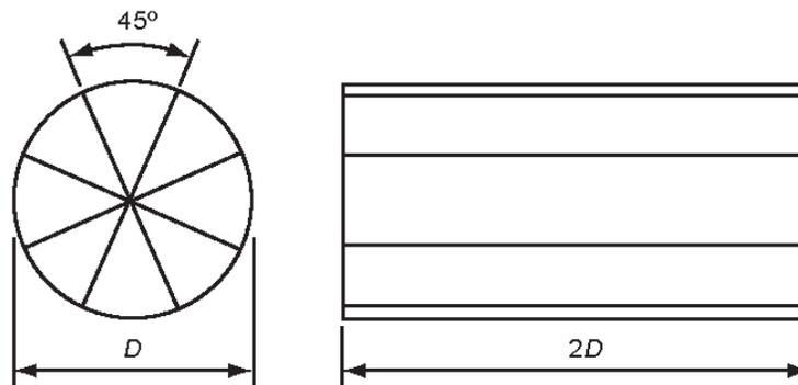
The star straightener will be constructed of eight radial blades of length equal to  $2D_4$  (with a  $\pm 1\%$  tolerance) and of thickness not greater than  $0.007D_4$ . The blades will be arranged to be equidistant on the circumference with the angular deviation being no greater than  $5^\circ$  between adjacent plates.
