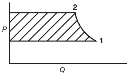
The fan output power ( $H_o$ ) is proportional to the shaded area which leads to:
