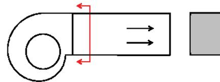
Fan outlet area for a centrifugal fan tested with an outlet duct is the gross cross-sectional area at the fan outlet, which is also equal to the test duct cross-sectional area, regardless of whether a cutoff plate is used to block a portion of the fan outlet.
