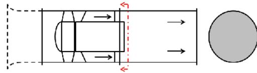
Fan outlet area for a ducted axial fan is the gross cross-sectional area at the fan outlet, which is also equal to the test duct cross-sectional area, regardless of whether the motor or inner shroud extends into the test duct.
