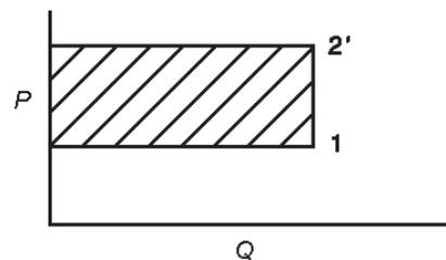
The fan output power is proportional to the shaded area, which leads to:
