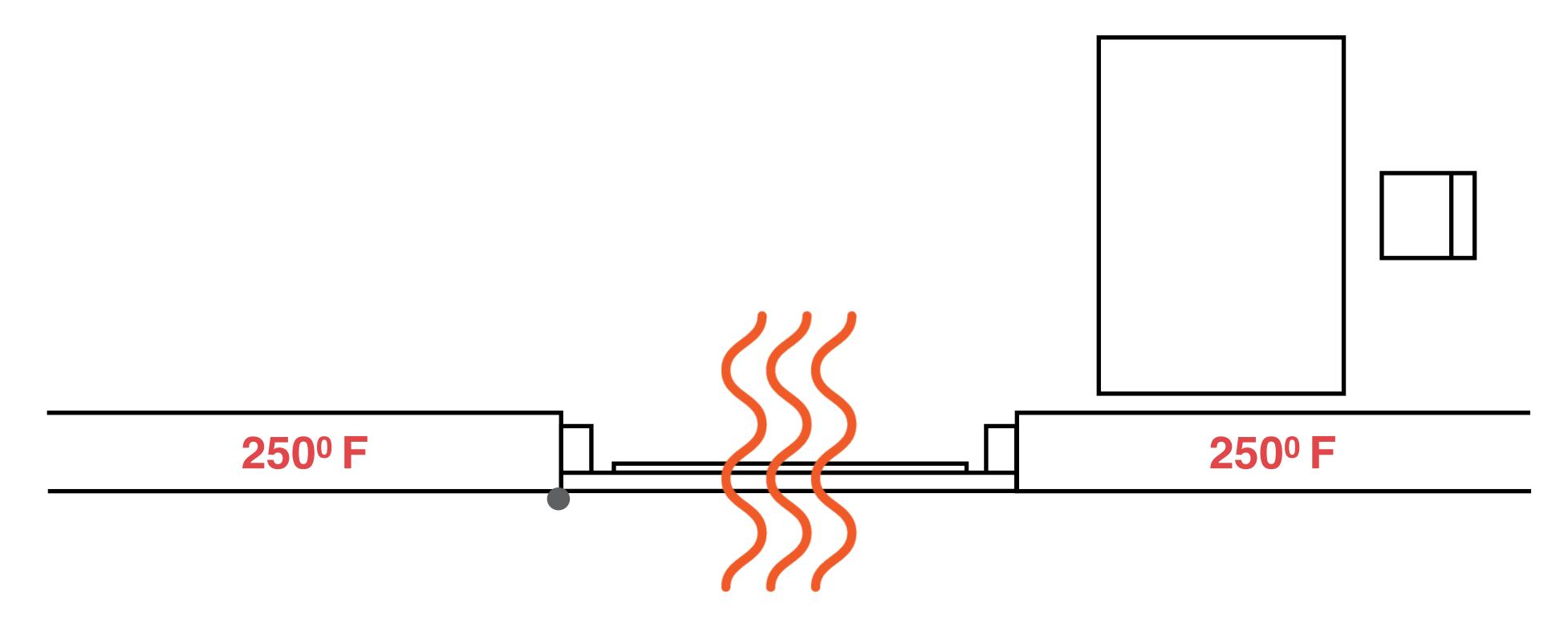
Fire-rated Doors – Tested for Flame-through and Flash-through ONLY
