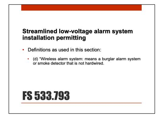
Many companies today utilize wireless systems. Systems that only plug directly into a receptacle, not unlike a toaster or an ipad. These operate on batteries that are of the low-voltage type either 1.5 volts, 3 volts, and 9 volt batteries.
