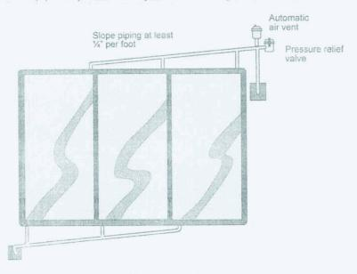
Figure 24 Piped and vented collector array
