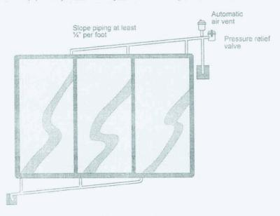
Figure 24 Piped and vented collector array
