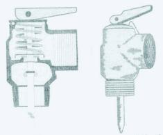
Figure 26 Pressure-temperature relief valve
