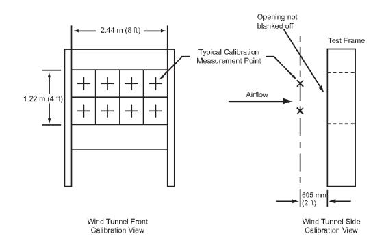
Figure 3 - Wind Stream Calibration Setup
