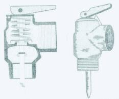
Figure 26 Pressure-temperature relief valve
