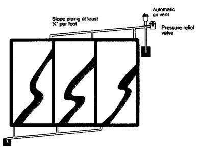
Figure 24 Piped and vented collector array
