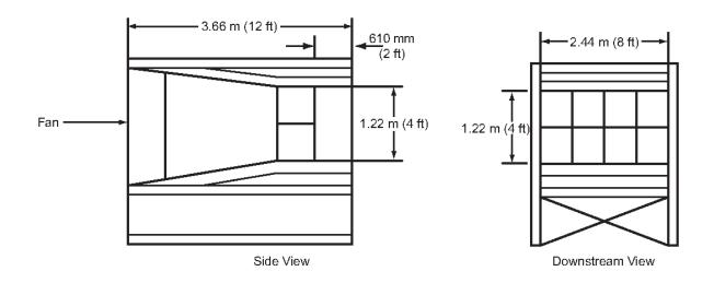
Figure 2 - Wind Tunnel with Baffles
