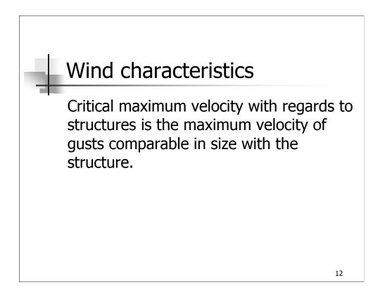
Wind can pulse building in resonance with natural frequency. Small amount of energy can induce almost unbounded deflections.
