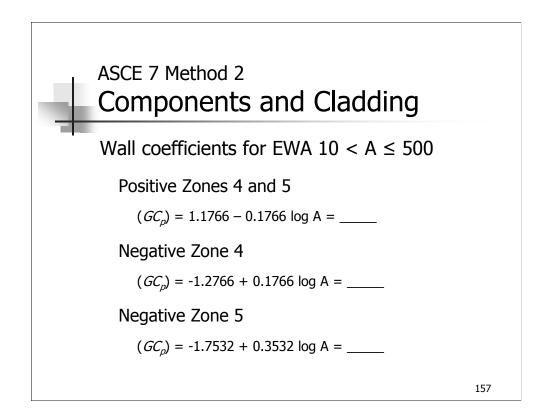
Note 5 in Figure 6-5a (page 231 in Appendix) states that pressure coefficients for walls can be reduced by 10% for buildings with roof slopes of 10 deg. or less.
