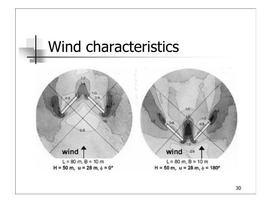
Configuration on right gives highest wind speed in passage *for given wind speed direction*.
