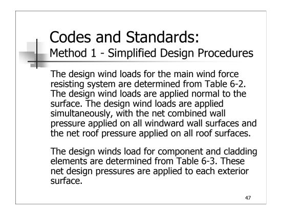
Method 1 has been added to the standard for a designer having the relatively common low-rise (h < 30 ft) regular shaped, simple diaphragm building case (see definitions for "simple diaphragm building" on the next slide) where pressures for the roof and walls can be selected directly from a table.
