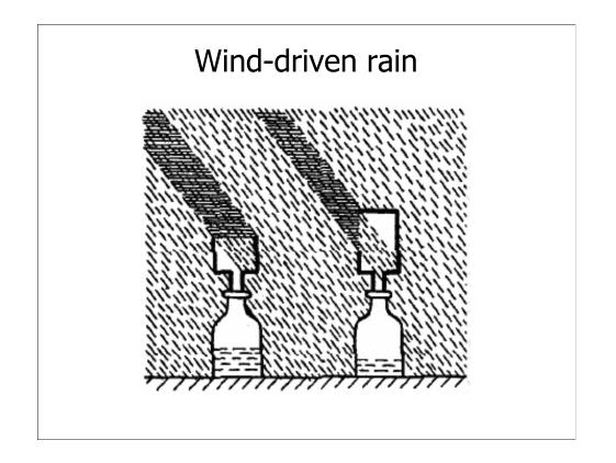
Test systems that measure the amount of rain entering an area from a vertical direction and a horizontal direction
