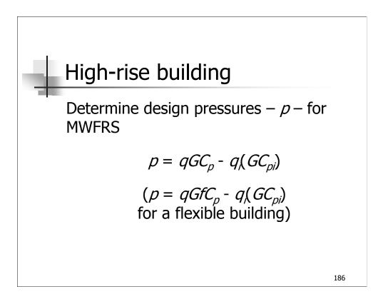
Design pressures are determined for each value of velocity pressure.
