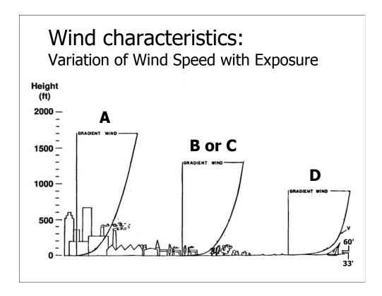
This graph illustrates the variations of wind speeds by height and exposure categories (exposure categories will be reviewed later). The velocity pressures will vary for both the Main Wind Force Resisting Systems and Components and Cladding by Exposure categories.
