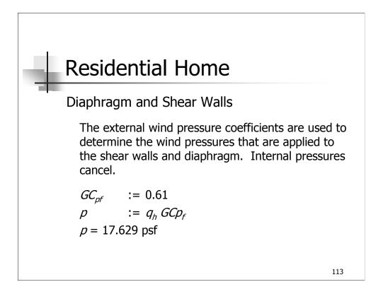
Typical calculation for determining design pressures.
