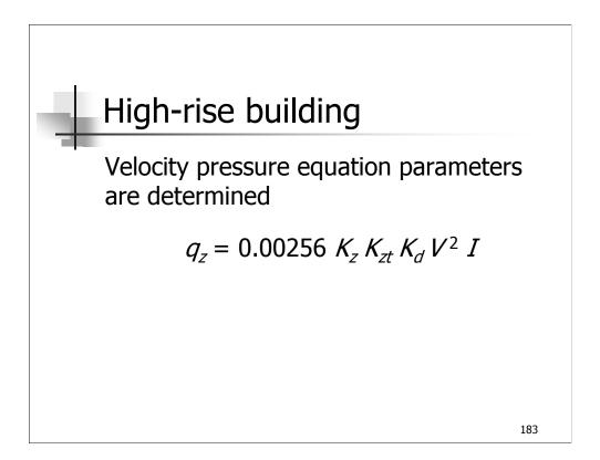
Velocity pressure equation from ASCE 7-98
