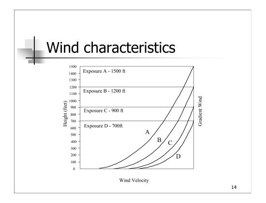
Wind Velocity Profiles and Boundary Layer Thickness
