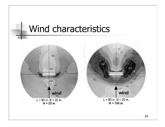
If building height is increased peak value of corners stay the same, size of corner stream increases.
