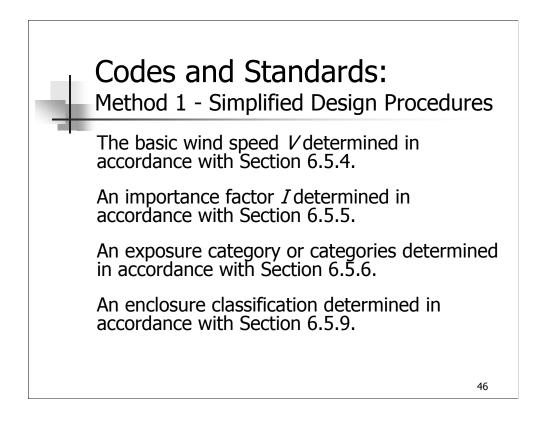
For the designer to use Method 1, the building must conform the all seven requirements in Section 6.4.1.
