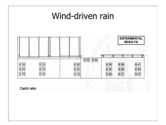
Results of measurements on test building. Ratios of rain collected at various positions on the building.
