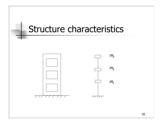
Three story building modeled as three degree of freedom structure for dynamic analysis. Mass of wall/columns divided and half added to floor above and half to floor below.
