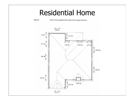
Shear forces applied to exterior walls
