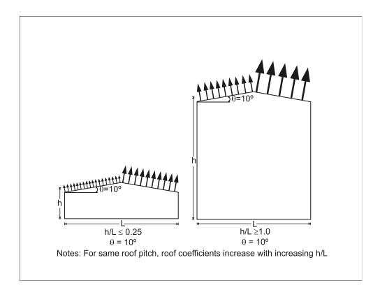
Graphical representation of Figure 6-3 of ASCE 7-98. Roof pitch less than or equal to 30 degrees.
