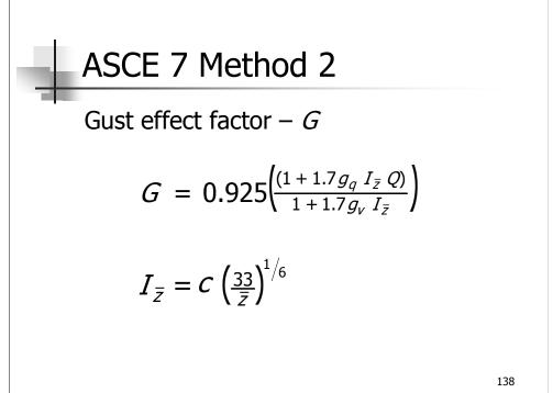
$I\overline{z}$  is intensity of turbulence at height  $\overline{z}$ .
