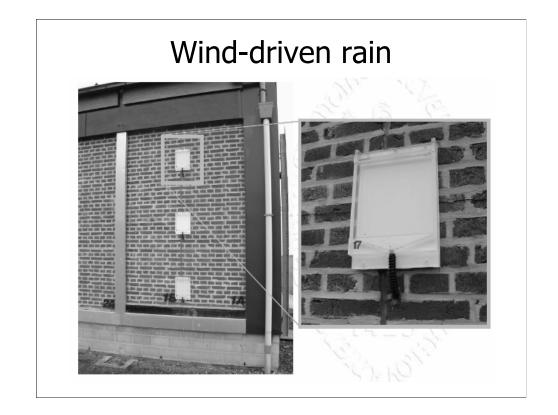
Rain measurement instruments mounted to the side of the test facility
