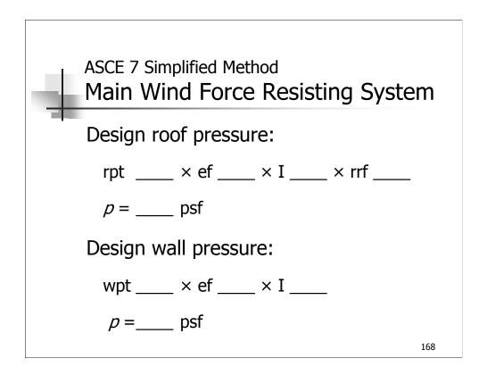
Design roof pressure acts uniformly over entire roof, includes internal pressure.
