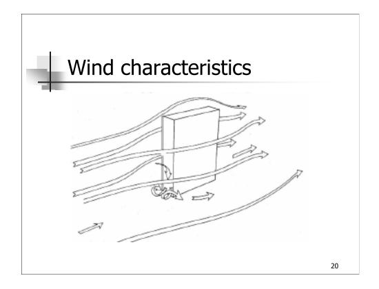
Wind flow around building. Arrows representing flow demonstrating turbulence at windward base of building and change in flow path as 'wind' encounters and goes around building.
