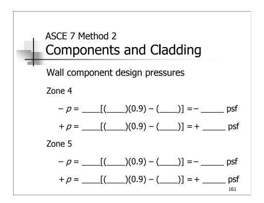
0.9 factor provides 10% reduction in external wall pressure coefficients, allowed because building roof pitch is less than 10 degrees.
