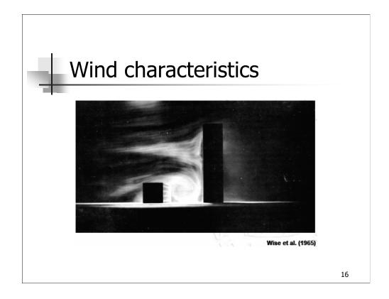
Note uplift induced on leeward side of windward building caused by vortex.
