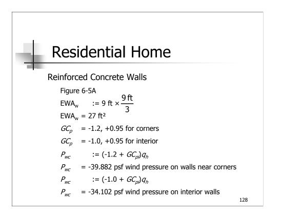
Effective Wind Area shall be taken as the span length multiplied by an effective width that need not be less than one-third the span length.
