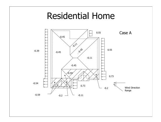
External pressure coefficients interpolated from Figure 6-4 for MWFRS Case A.
