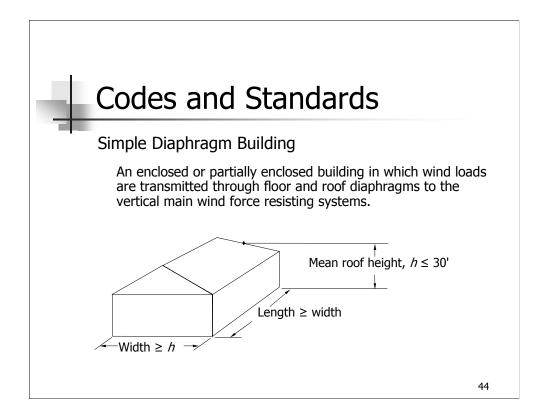
Definition for *Building, Simple Diaphragm* as found in ASCE 7-98: An enclosed or partially enclosed building in which wind loads are transmitted through floor and roof diaphragms to the vertical main wind force resisting systems.
