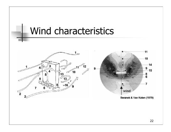
Results of research undertaken to investigate 'problem' wind caused by accelerations around buildings. Directed at finding ways to alleviate pedestrian annoyance, it also shows interaction of wind/buildings.
