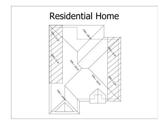
Effective Wind Area of pre-engineered roof trusses.
