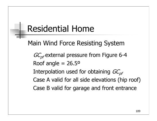
Case A valid for all side elevation because building has hip roof.
