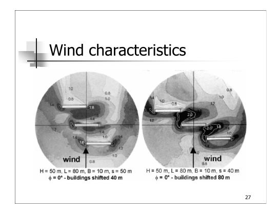
Highest wind speed through passages in right side configuration.
