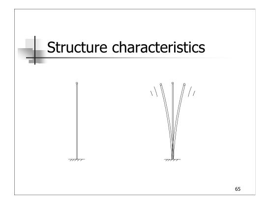
'Pluck' a flagpole and it vibrates at natural frequency. First mode fundamental frequency shown.
