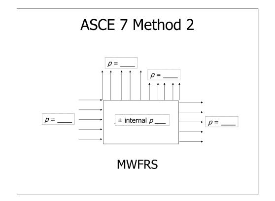
Pressures on windward and leeward walls and along roof for 30 foot length.
