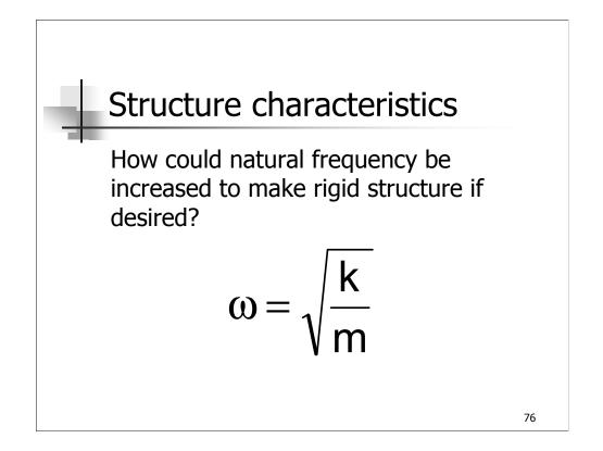
First mode natural frequency is 0.718 Hz, therefore it is a flexible structure. To increase natural frequency either increase column stiffness or reduce mass.
