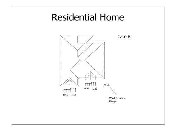
External pressure coefficients interpolated from Figure 6-4 for MWFRS Case B.
