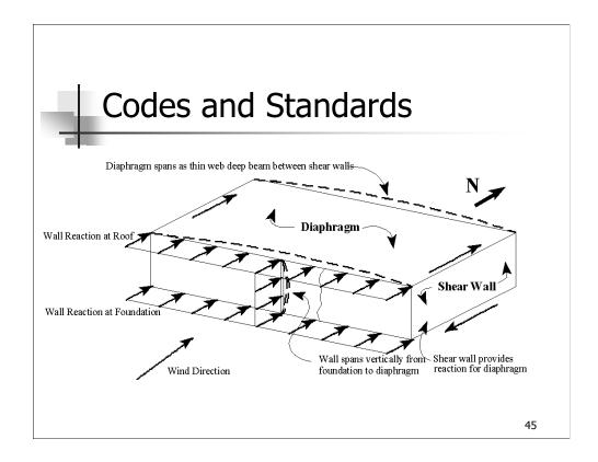
Building demonstrating 'diaphragm' action from wind loading
