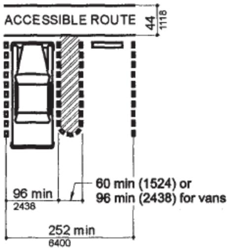
502.3 Access Aisle. Access aisles serving parking spaces shall comply with 502.3. Access aisles shall adjoin an accessible route. Two parking spaces shall be permitted to share a common access aisle. Parking access aisles must be part of an accessible route to the building or facility entrance. Access aisles must be placed adjacent to accessible parking spaces.
