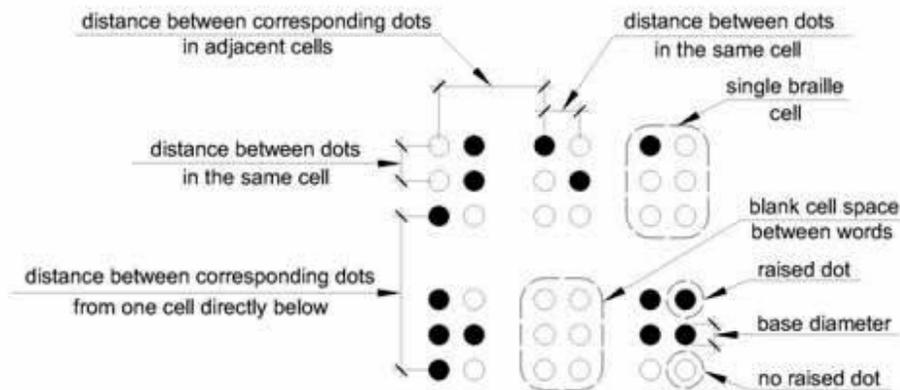
**Figure 703.3.1 Braille Measurement**
