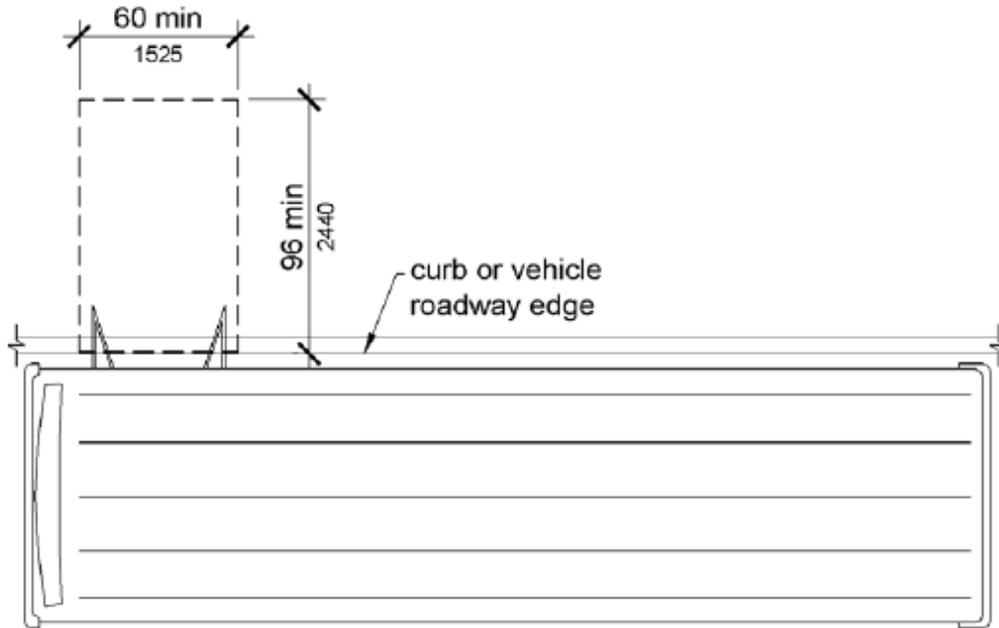
**Figure 810.2.2 Dimensions of Bus Boarding and Alighting Areas**
