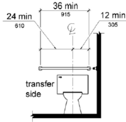
Figure 604.5.2 Rear Wall Grab Bar at Water Closets
