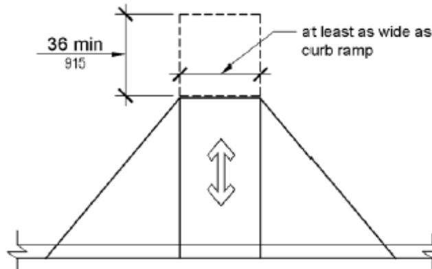
**Figure 406.4 Landings at the Top of Curb Ramps**
