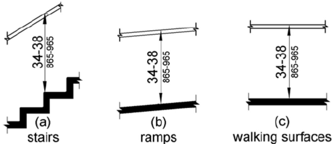
Figure 505.4 Handrail Height
