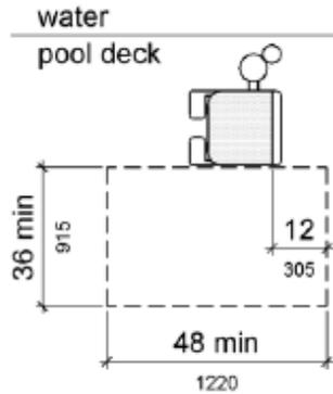
Figure 1009.2.3 Clear Deck Space at Pool Lifts
