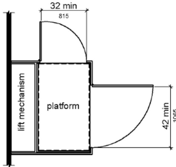
Figure 410.6 Platform Lift Doors and Gates
