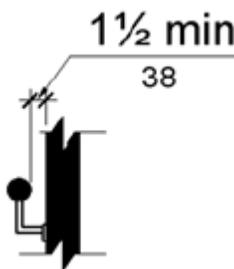
Figure 505.5 Handrail Clearance
