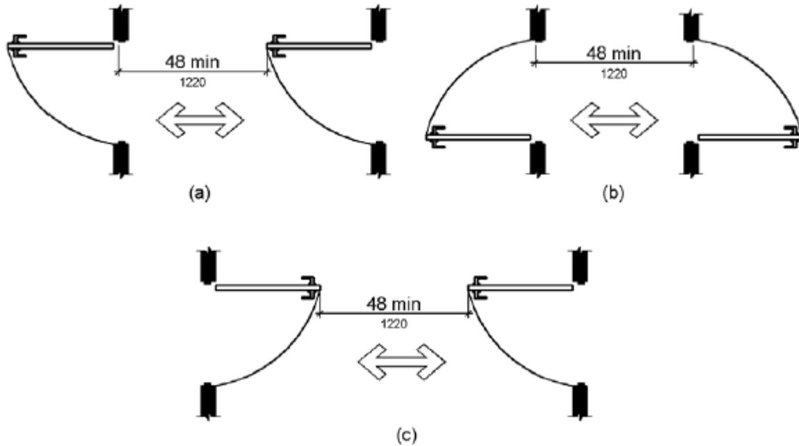
**Figure 404.2.6 Doors in Series and Gates in Series**
