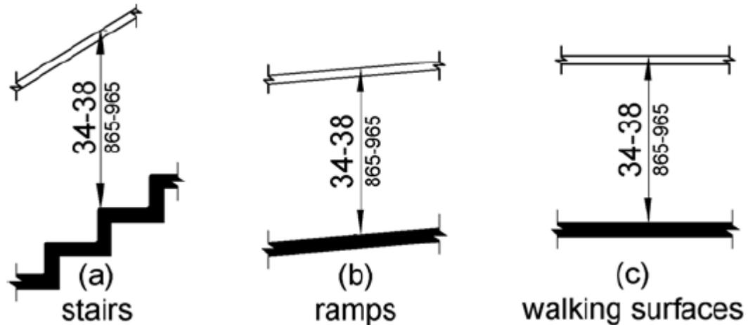
Figure 505.4 Handrail Height
