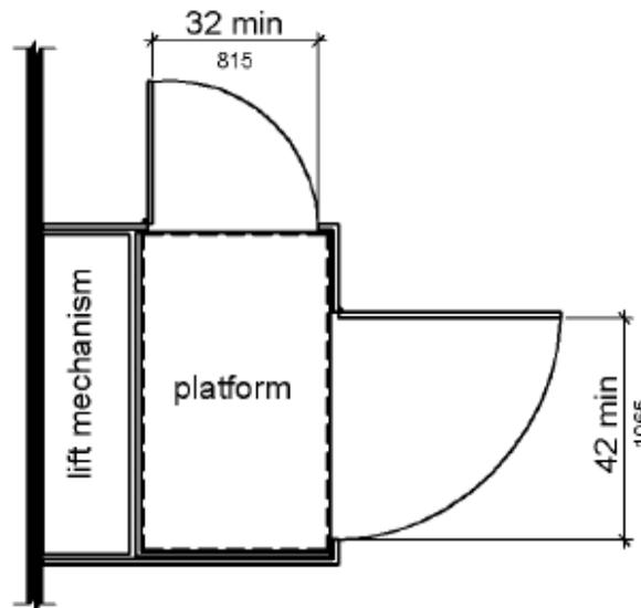
**Figure 410.6 Platform Lift Doors and Gates**
