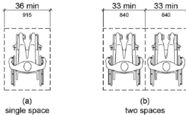
**Figure 802.1.2 Width of Wheelchair Spaces in Assembly Areas**
