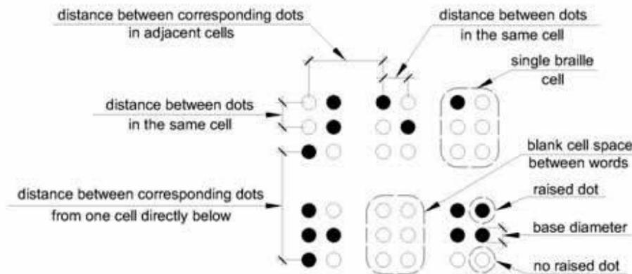
**Figure 703.3.1 Braille Measurement**
