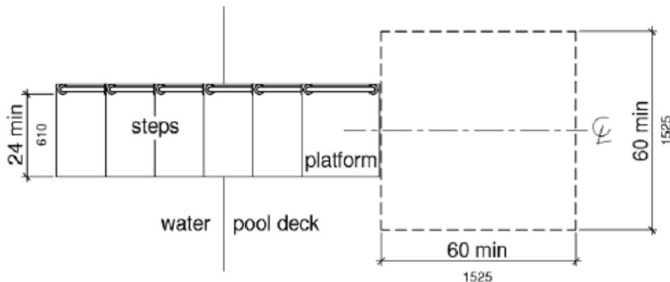
Figure 1009.5.2 Clear Deck Space at Transfer Platform
