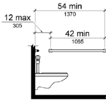
**Figure 604.5.1 Side Wall Grab Bar at Water Closets**
