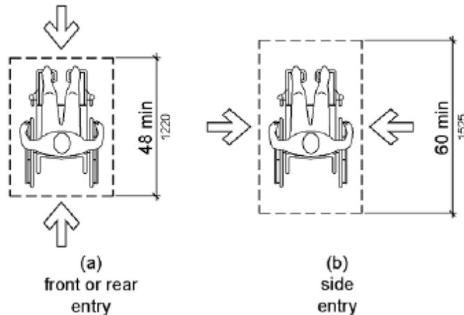
**Figure 802.1.3 Depth of Wheelchair Spaces in Assembly Areas**
