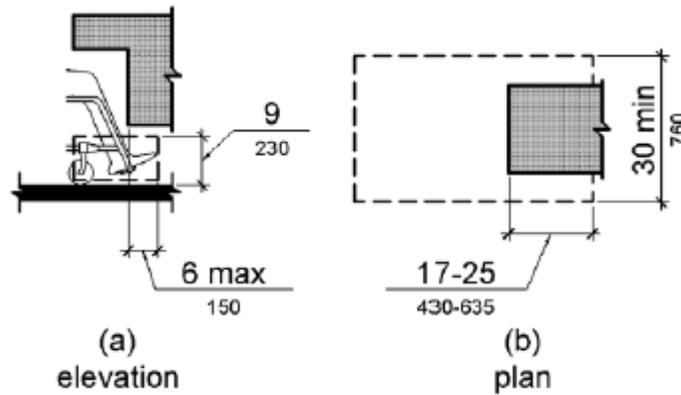
Figure 306.2 Toe Clearance
