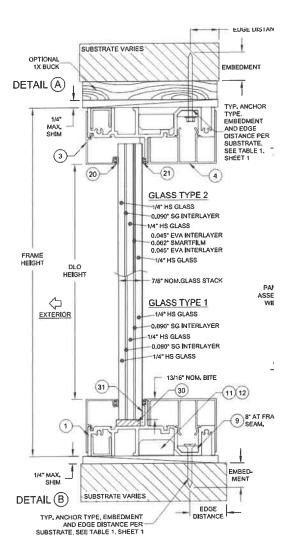
4) The glass used in FL #15709 is triple laminated glass - 1/4"HS + 0.090"SG + 1/4"HS, the total glass thickness is 0.837", the glass capacity as per FL#15709 is 90 psf
