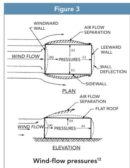
produces suction or outward pressures on sidewalls, the leeward wall and, depending on geometry, the roof.
