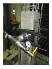
Figure 4. Carbonation Chamber
