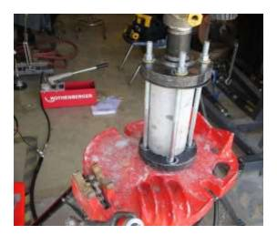
Figure 17. Water Pressure Drop Concrete Test Apparatus
