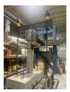
Figure 8. Picture of Column Setup for Accelerated Carbonation under Axial Loading
