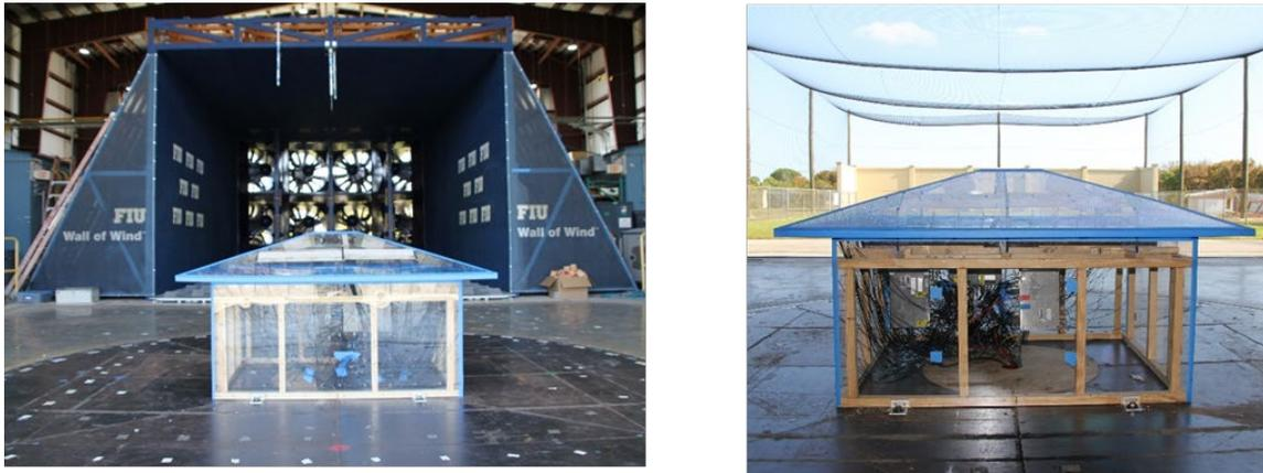
Figure 8 Model B Configuration on the turntable at the Wall of Wind.
