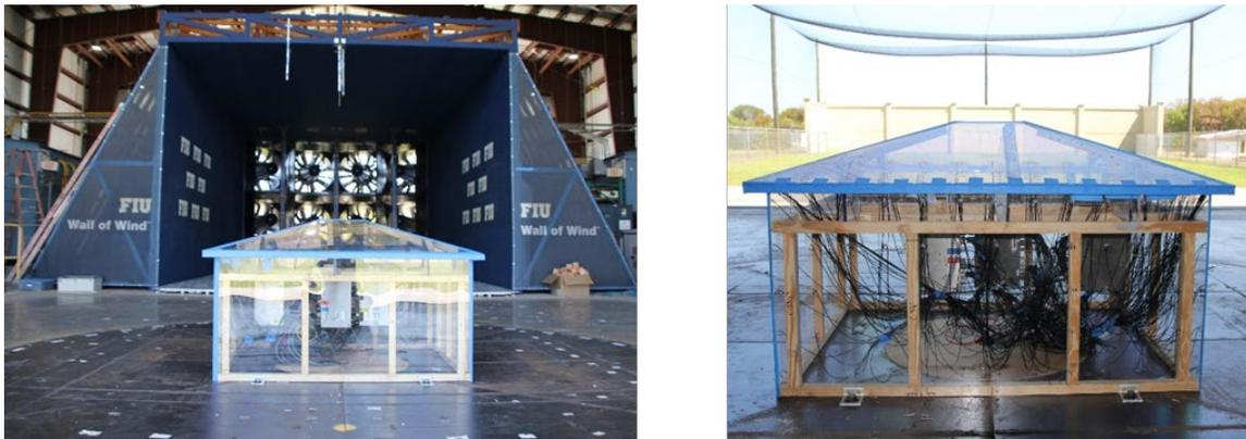
Figure 6 Model A Configuration on the turntable at the Wall of Wind.
