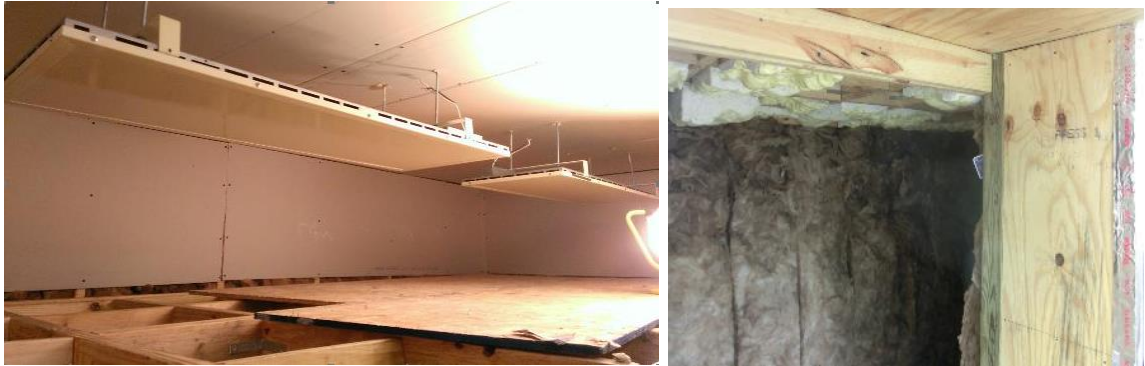
Figure 16: Thermally controlled top portion (Left) lower interior chamber open to ambient Temperature (Right).
