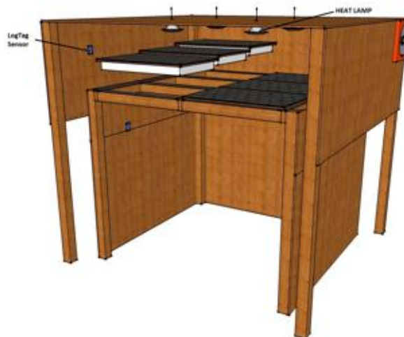
Figure 14: Isometric view of Insulated Thermal Chamber
