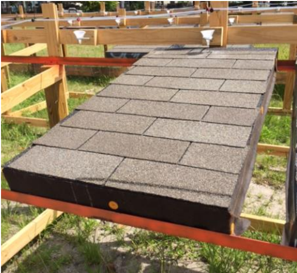
Figure 31: Membrane installed on all edges to prevent uncontrolled moisture travel
