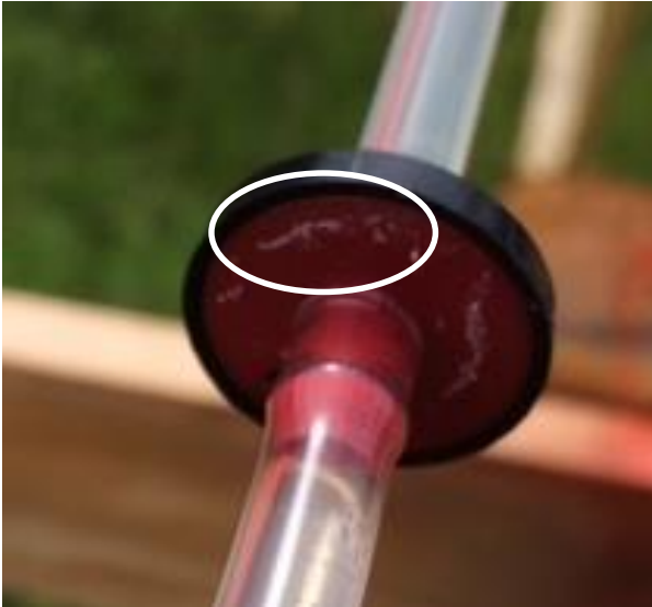
Figure 35: Old dripper with mineral deposits indicated by white ellipse
