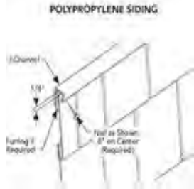
Figure R703.14.1.1.2 (1) Typical Trim Under Window and Top of Walls Polypropylene Siding
