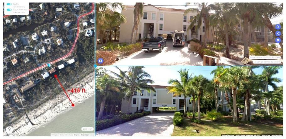
Illustrative effect of the vegetation and extended setback in Sanibel potentially mitigating surge impacts to structures. Subset (a) provides the post-storm aerial view showing a setback of approximately 415 ft from the shoreline, (b) the post-storm surface-level view, and (c) the pre-storm surface-level view.
