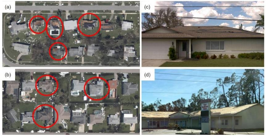
Illustrative performance of asphalt shingle and rolled membrane roofs in Port Charlotte consisting of homes constructed in the (a) 1960s with asphalt shingles and rolled roofs, (b) 1980s, (c) 1980s construction but asphalt shingle roof installed in 2005 but also (d) isolated commercial structures.
