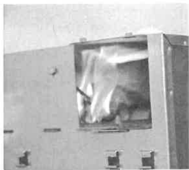
The impeller has ignited and begins to sag onto the motor
