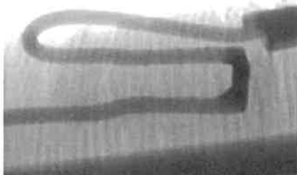
Radiograph of the fusible link
