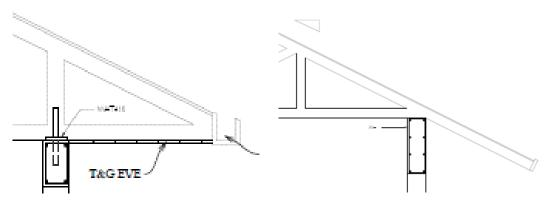
Figure 1. Structural detail of overhang with and without a soffit.
