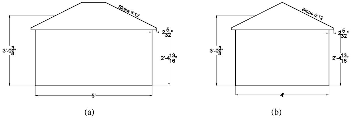
Figure 2 Configuration B model layout (a) Elevation View (b) Side View
