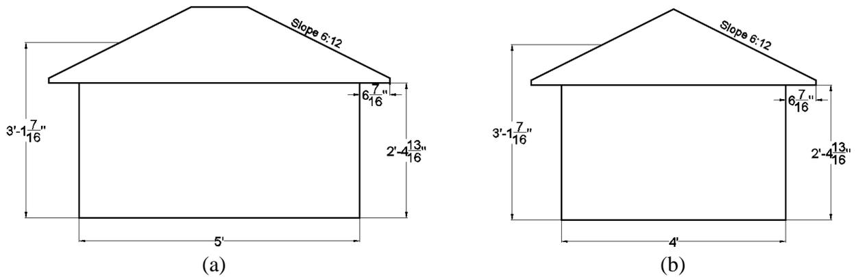
Figure 4 Configuration D model layout (a) Elevation View (b) Side View
