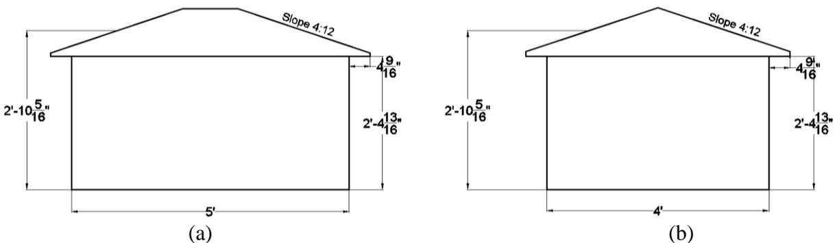
Figure 1 Configuration A model layout (a) Elevation View (b) Side View
