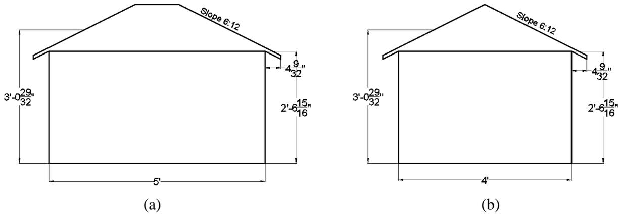
Figure 6 Configuration F model layout (a) Elevation View (b) Side View
