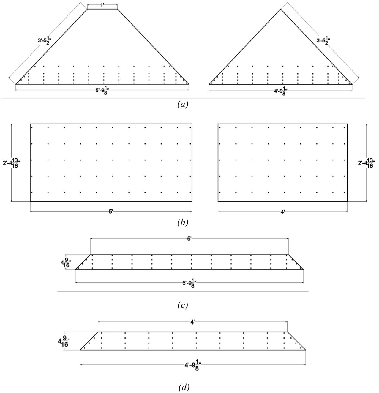
Figure 7 Pressure taps instrumentation on configuration A model (a) Roof (b) Longitudinal and Side Walls (c) Longitudinal overhang (d) Side overhang
