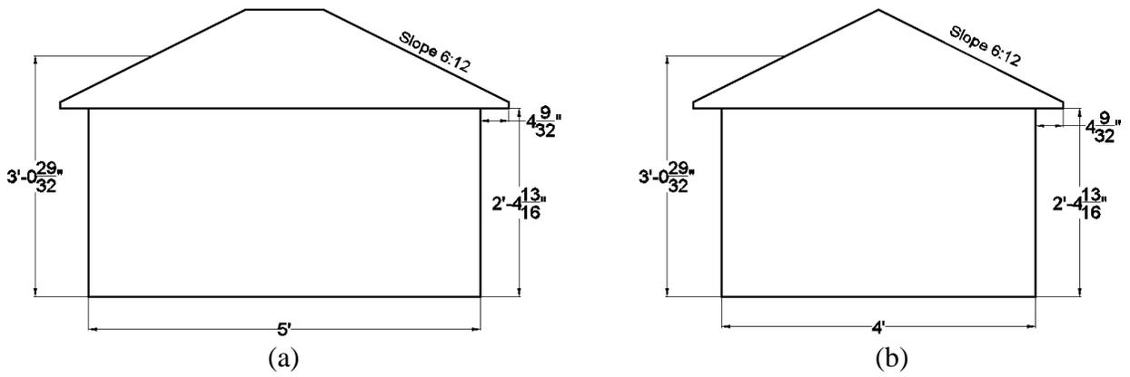
Figure 3 Configuration C model layout (a) Elevation View (b) Side View
