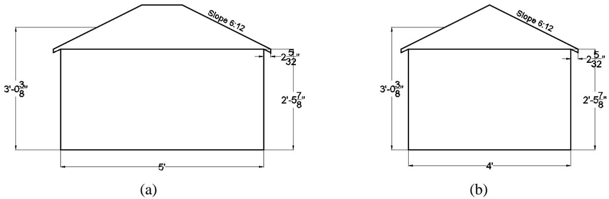
Figure 5 Configuration E model layout (a) Elevation View (b) Side View
