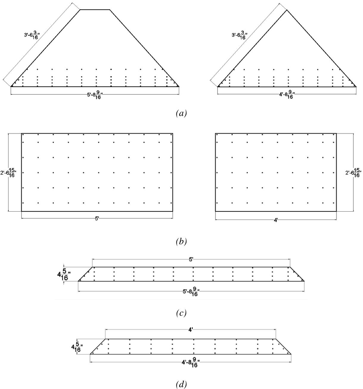
Figure 12 Pressure tap instrumentation on configuration F model (a) Roof (b) Longitudinal and Side Walls (c) Longitudinal overhang (d) Side overhang
