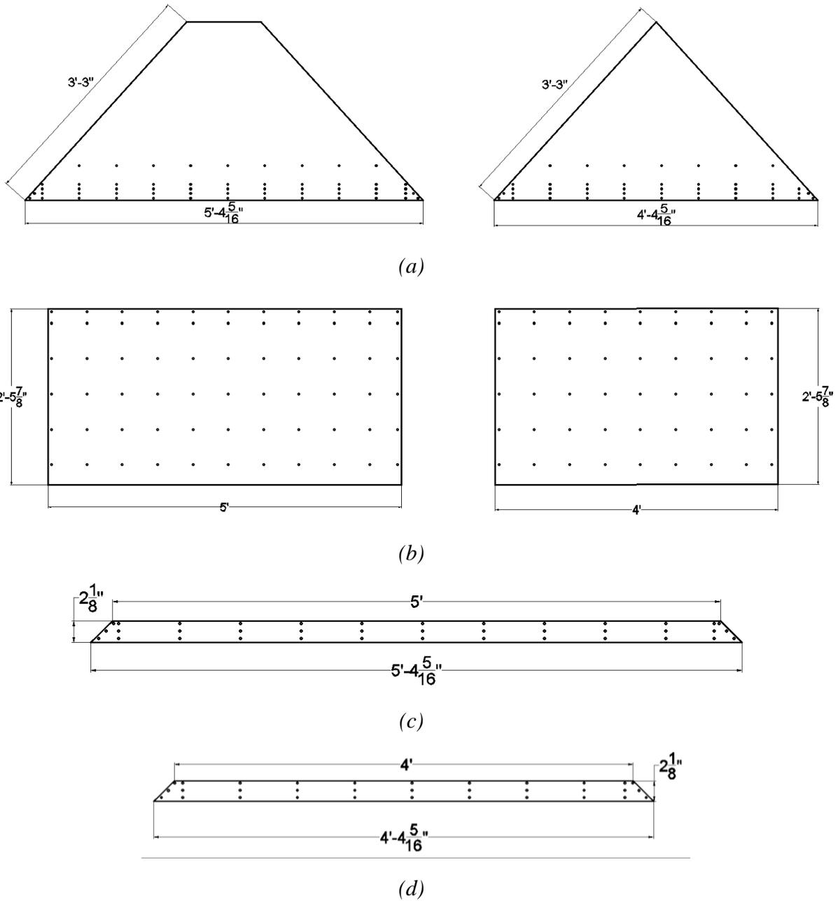
Figure 11 Pressure taps instrumentation on configuration E model (a) Roof (b) Longitudinal and Side Walls (c) Longitudinal overhang (d) Side overhang
