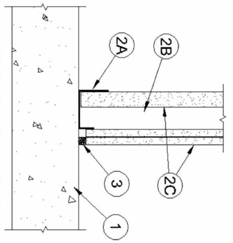
1. Floor Assembly — Min 4-1/2 in. (114 mm) thick reinforced lightweight or normal weight (100-150 pcf or 1600-2400 kg/m³) structural concrete. Floor may also be constructed of any min 6 in. (152 mm) thick UL Classified hollow-core Precast Concrete Units\*.
