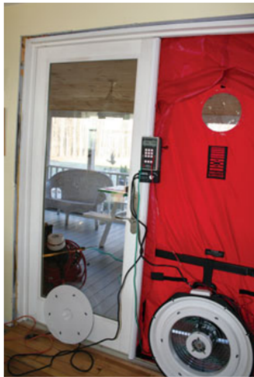
Figure 3: Blower Door Test
