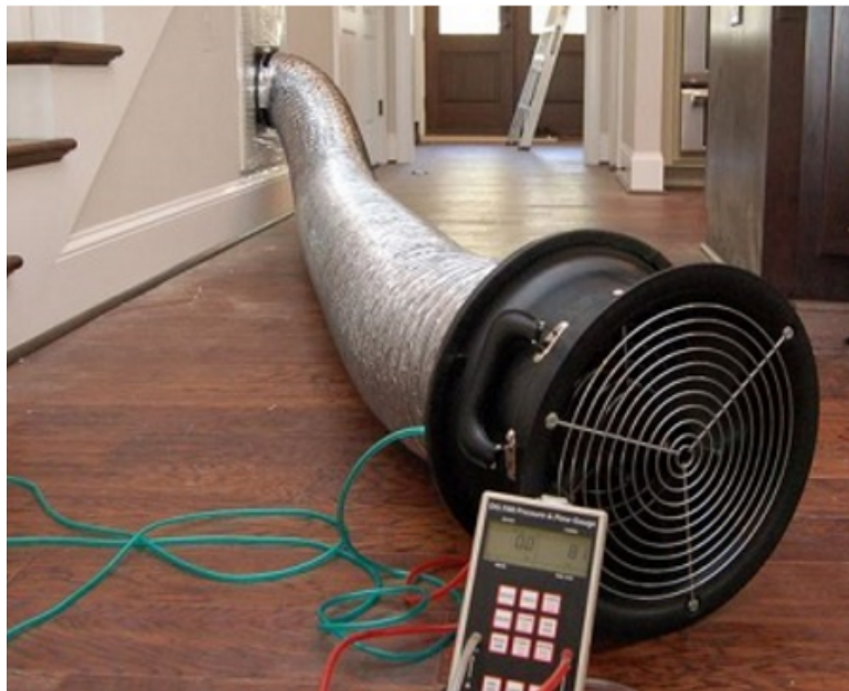
Figure 4. Minneapolis Duct Blaster System
