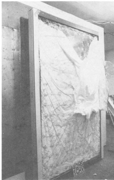
FIG. 8. Tearing of Laminate for Heat-Strengthened Laminated Glass
