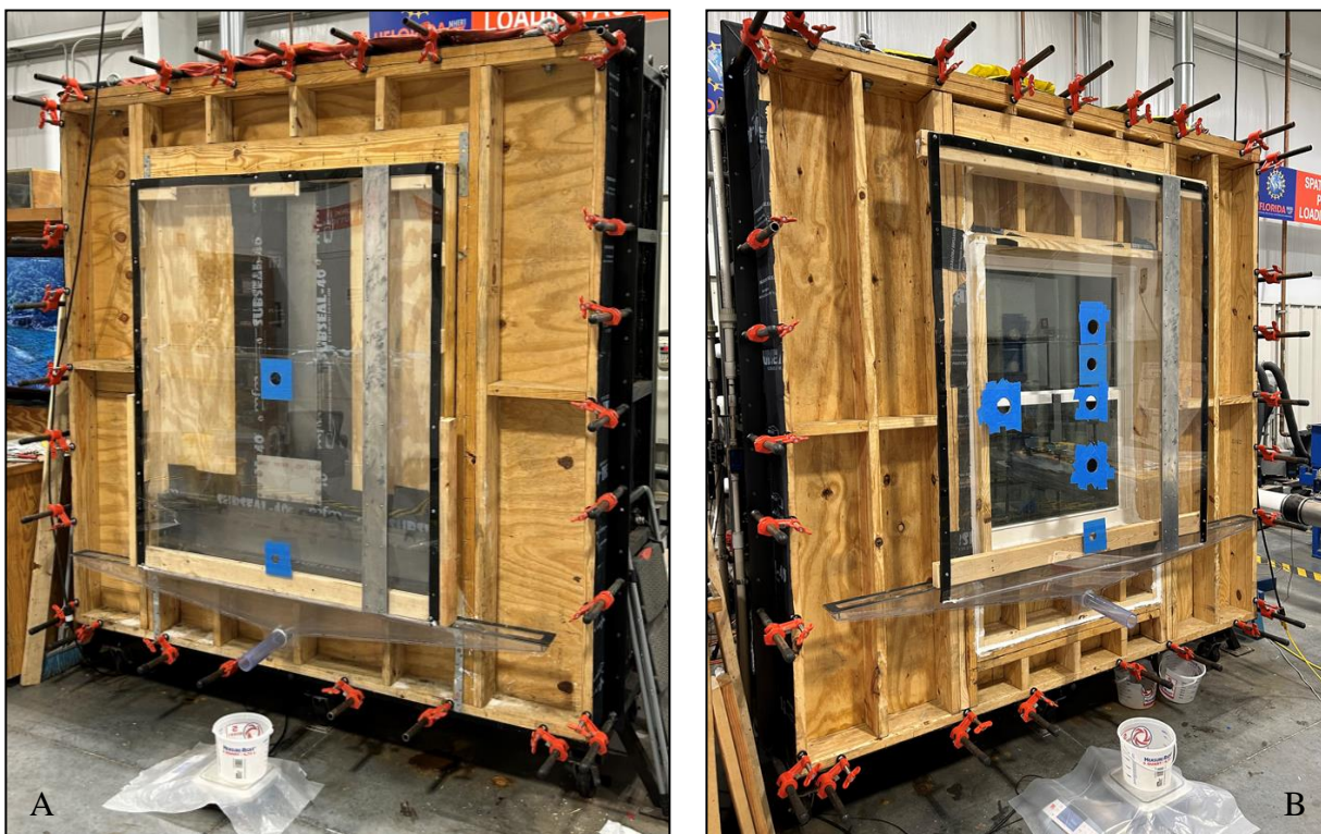
Figure 1. UF HAPLA experimental setup with wood stud-framed wall unit: A) Round 1 test specimen; and B) Round 2 test specimen.
