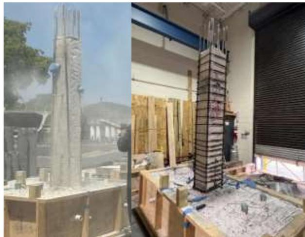
Figure 24. Column Sandblasting and Shell Retrofit
