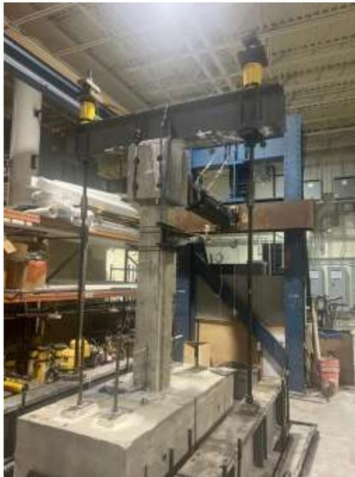
Figure 8. Picture of Column Setup for Accelerated Carbonation under Axial Loading
