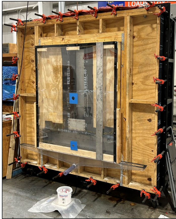
Figure 1. HAPLA with timber frame wall unit and installed Round 1 test specimen.
