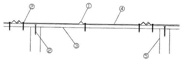
1. Metal Roof Deck Panels\* — No. 29 MSG min thick coated steel. 24 in. cover width (26 in. overall width). AMERICAN CONSTRUCTION METALS (View Classification) — "5V Crimp"
