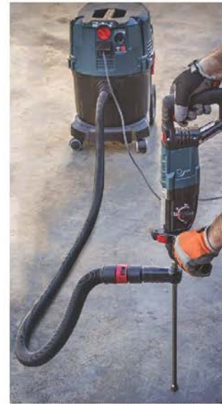
Bosch / Simpson Strong-Tie DXS drill bit used with the vacuum dust extraction system described in Section 3.2.3.2
