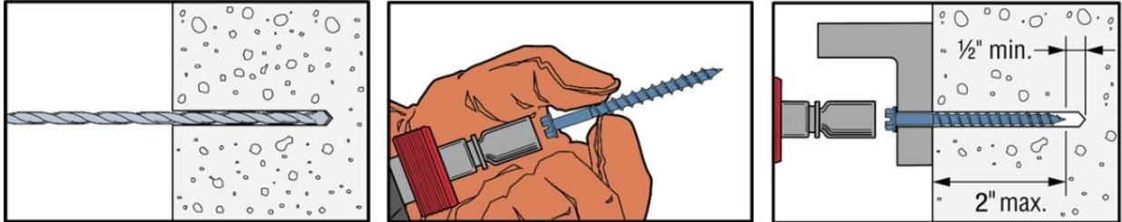
Figure 2 – Installation Instructions for Titen Turbo™ Screw Anchors
