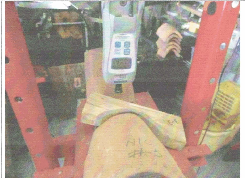
Specimen #5 Ultimate Load: 377.4 lbs.
