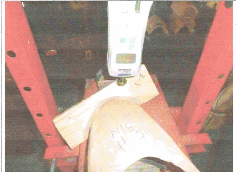
Specimen #3 Ultimate Load: 445.6 lbs.
