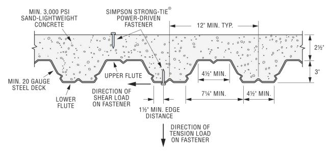
FIGURE 9—INSTALLATION IN 21/2-INCH CONCRETE FILL OVER 3-INCH-DEEP STEEL DECK
