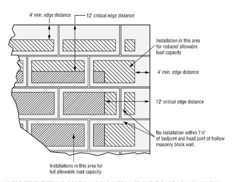
FIGURE 4—STAINLESS STEEL TITEN HD SCREW ANCHOR INSTALLED IN THE FACE OF HOLLOW CMU (CONCRETE MANSORY UNIT) WALL CONSTRUCTION (Refer to Table 5, 6 and 7)
