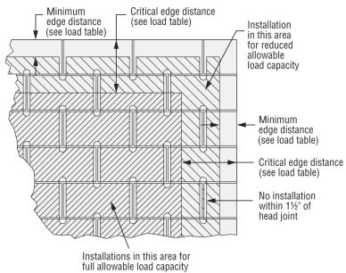
FIGURE 2—CARBON STEEL AND STAINLESS STEEL TITEN HD SCREW ANCHOR INSTALLED IN THE FACE OF GROUT-FILLED CMU (CONCRETE MANSORY UNIT) WALL CONSTRUCTION (Refer to Table 1, 2, and 3)
