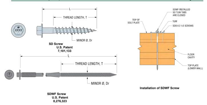
FIGURE 1—SD AND SDWF SCREWS
