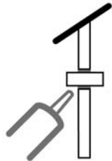
4. Sealant at penetrations
