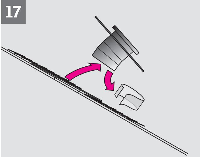
**ENGLISH:** Remove flashing with elbow and remove protective film from upper elbow.
