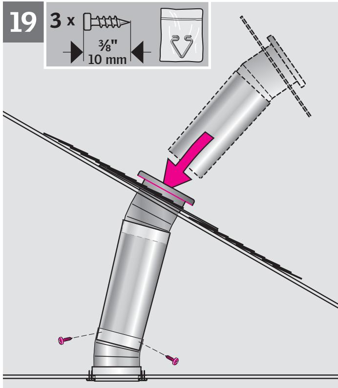
**ENGLISH:** Connect tunnel assembly with the clips supplied. If tunnel section was trimmed or holes do not align, use the screws supplied.
