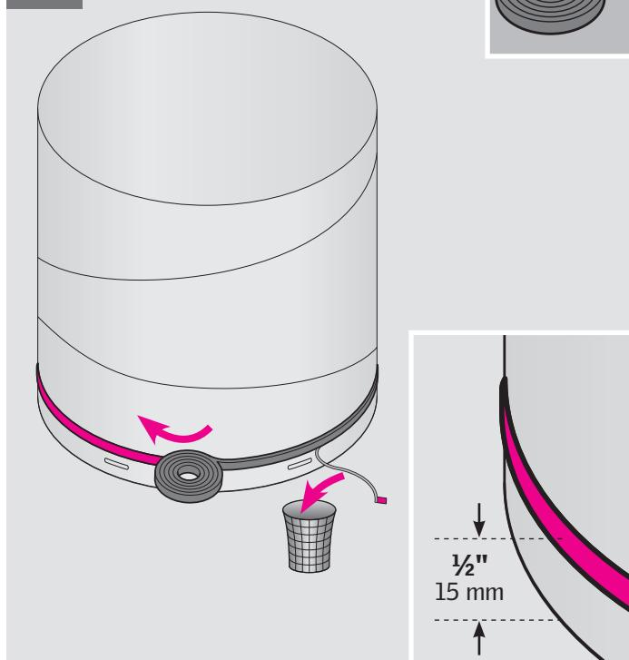
**ENGLISH:** Attach pile gasket to lower elbow as shown.
