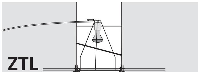
**ENGLISH:** Install the trim ring by aligning notches and rotate to secure.
