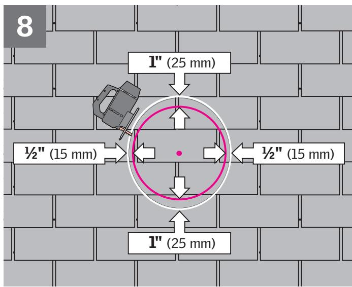
**ENGLISH:** Mark and cut a rough opening of  $\frac{1}{2}$ " (15 mm) outside the circle at sides and 1" (25 mm) outside the circle at top and bottom.
