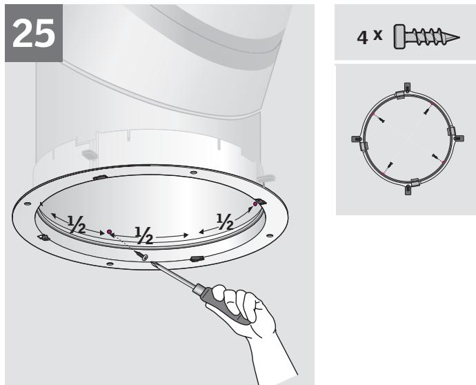
**ENGLISH:** Secure tunnel assembly to ceiling ring with four of the  $\frac{3}{8}$ " (10 mm) screws provided.
