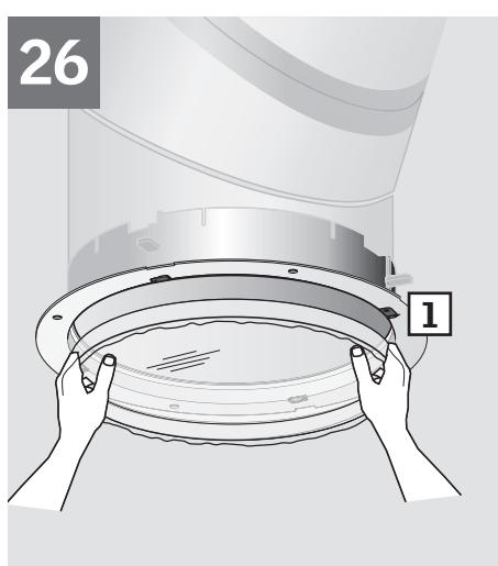
**ENGLISH:** Install the diffuser with the frosted side facing down. Secure the diffuser by rotating the plastic locks into locked position **1**.
