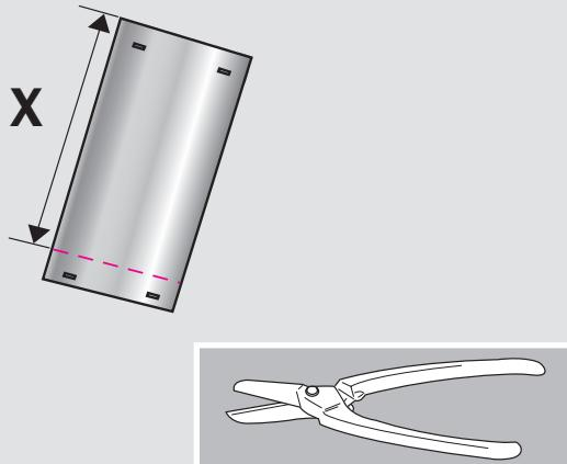
**ENGLISH:** If necessary, cut the rigid tunnel section to length **A**. Additional tunnel sections can be overlapped to form a telescoping tunnel section. Secure joints with two of the  $\frac{3}{8}$ " (10 mm) screws **B**.
