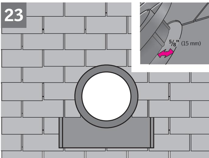
**ENGLISH:** Reinstall roofing material over the flange. Leave a  $\frac{5}{8}$ " (15 mm) channel for water to run off.
