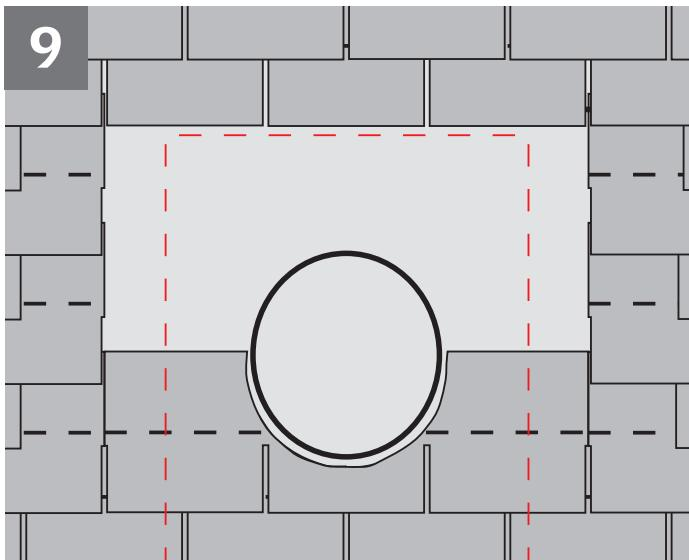
**ENGLISH:** Remove the roofing material around the upper half of the rough opening as indicated.
