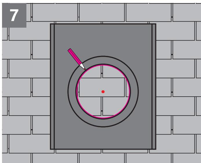
**ENGLISH:** Locate the nail indicating the center of the sun tunnel on the roof and use the flashing to mark a circle.
