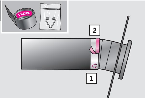
**ENGLISH:** Connect the rigid tunnel section with upper elbow, fitting the rigid tunnel section to go on the outside of the upper elbow. Secure and tape joints with tunnel clips and tape provided **1, 2**.
