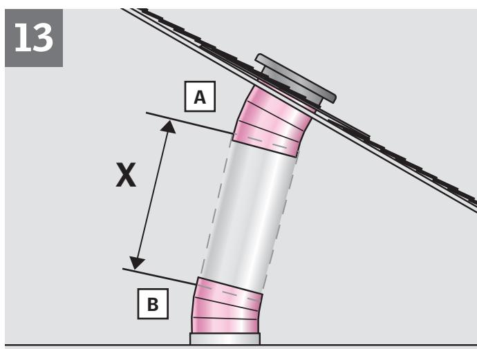
**ENGLISH:** Adjust the angle of both elbows so that they point directly against each other **A**, **B**. Elbows can be damaged if excess force is applied.
