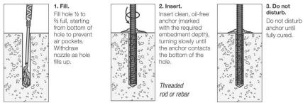
Note: Refer to Table F for proper gel times and cure times and Table D and E for maximum tightening torgue. Nozzle extensions may be needed for deep holes.
