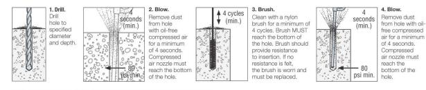
Note: Refer to Tables A, B, and C for proper drill bit size and brush part number.
