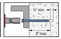
Figure 2 – Installation Instructions for Titen Turbo $^{\text{TM}}$  Screw Anchors
