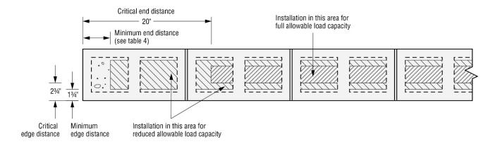
FIGURE 3A –½ INCH AND % INCH DIAMETER THREADED ROD ALLOWABLE ANCHOR LOCATIONS FOR FULL AND REDUCED LOAD CAPACITY WHEN INSTALLATION IS IN THE TOP OF FULLY GROUTED CMU MASONRY WALL CONSTRUCTION
