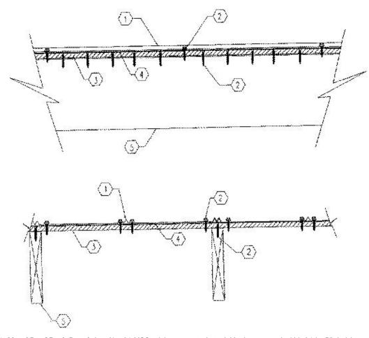
1. **Metal Roof Deck Panels\*** — No. 26 MSG minimum coated steel. Maximum panel width 24 in. Rib height maximum 1/2 in. Panels continuous over two or more spans. A bead of sealant may be used at panel sidelaps.
