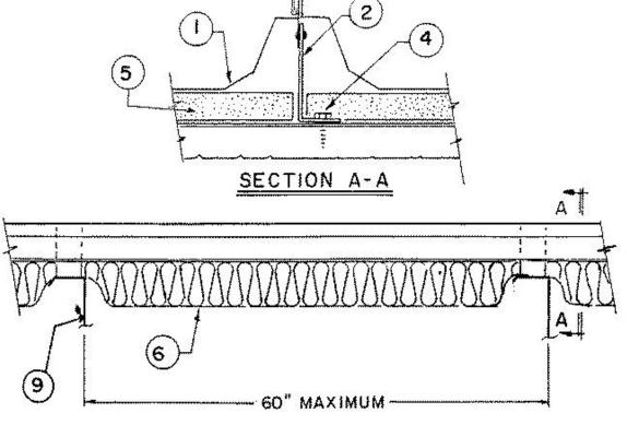
1. Metal Roof Deck Panels\* — For class 90-No. 24 MSG coated steel, for class 30-No. 26 MSG min. Coated steel, steel. Panels continuous over two or more spans. End laps to occur adjacent to purlins with panels overlapped 3 inch max. A line of sealant may be used at panel end and side laps.
