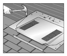
**4. SECURE** vent at 4-inch centers using roofing nails of sufficient length to penetrate sheathing. **SEAL** all penetrations using locally-approved sealant (Class A where required by code for flame resistance).
