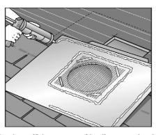
**2. SEAL** using sufficient amount of locally-approved sealant (Class A where required by code for flame resistance) around inner and outer flange.
