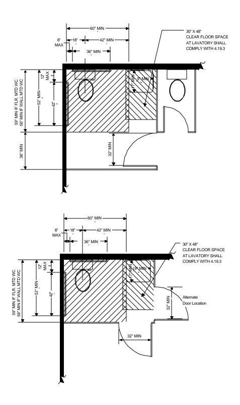
IN NEW CONSTRUCTION, A LAVATORY SHALL BE PROVIDED WITHIN THE ACCESSIBLE TOILET STALL. THE LAVATORY SHALL NOT ENCROACH INTO THE REQUIRED CLEAR FLOOR SPACE FOR THE WATER CLOSET.
