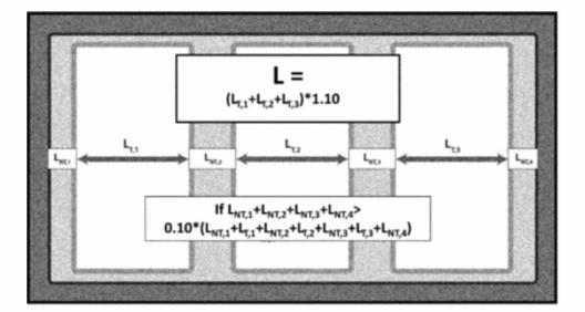
Figure A3.5 Three-door vertical closed transparent display case, where the distance "L" is the collective length of portions of the merchandiser through which product can be seen, including the linear dimension of transparent ( $L_{T,i}$ ) and non-transparent ( $L_{NT,i}$ ) areas, and the total linear dimension of non-transparent areas is greater than 5 inches.
