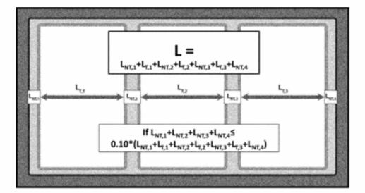
Figure A3.4 Three-door vertical closed transparent display case, where the distance "L" is the collective length of portions of the merchandiser through which product can be seen, including the linear dimension of transparent ( $L_{T,i}$ ) and non-transparent ( $L_{NT,i}$ ) areas, provided the total linear dimension of non-transparent areas are less than 5 inches.
