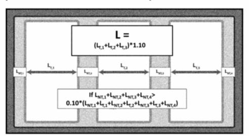
Figure A3.5 Three-door vertical closed transparent display case, where the distance "L" is including the linear dimension of transparent ( $L_{T,i}$ ) and non-transparent ( $L_{NT,i}$ ) areas, and the total linear dimension of non-transparent areas is greater than 5 inches.
