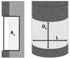
Figure A3.3 Radius case, where the distances " $D_h$ " and "L," and the area " $A_e$ ," are representative of the planar projections of visible product when viewed at an angle normal to the transparent surface or opening.
