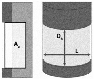
Figure A3.3 Radius case, where the distances " $D_h$ " and "L," and the area " $A_e$ ," are representative of the planar projections of visible product when viewed at an angle normal to the transparent surface or opening.
