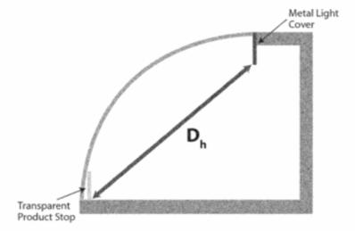
Figure A3.2 Service over counter display case, the distance " $D_h$ " is the dimension of the projected visible product, that being the dimension transverse to the length of the case through which product can be viewed, excluding areas of the product zone that cannot be viewed as part of a direct projection through the glass front.
