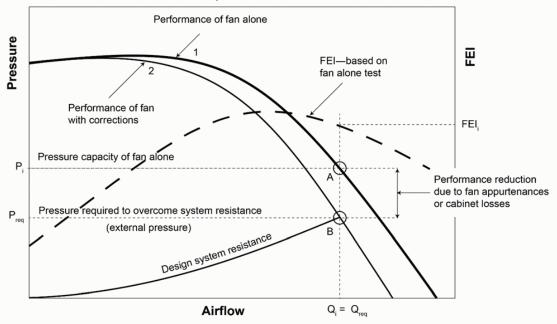
Figure 1-Fan Curves at Constant RPM and Blade Pitch
