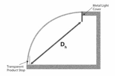
Figure A3.2 Service over counter display case, the distance " $D_h$ " is the dimension of the projected visible product, that being the dimension transverse to the length of the case through which product can be viewed, excluding areas of the product zone that cannot be viewed as part of a direct projection through the glass front.
