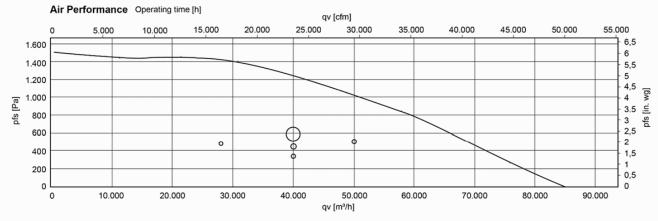
The fan combination selected in the results list is displayed as a characteristic curve at maximum modulation. The specified operating points are also shown; the size of the points represents the proportional operating duration.
