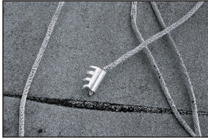
Figure 7. A failed prong-type splice connector. If conductors become detached from the roof, they are likely to pull from pronged splice connectors.
