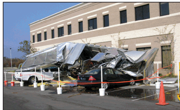
Figure 2. This 30' x 10' x 8' 18,000-pound HVAC unit was attached to its curb with 16 straps (one screw per strap). Although the wind speeds were estimated to be only 85 to 95 miles per hour (3-second peak gust), it blew off the building.
