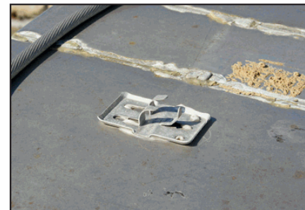
Figure 3. During high winds, the conductor deformed the prongs and pulled away from this conductor connector.
