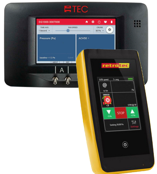
Figure 2. Digital pressure gauges from The Energy Conservatory and, inset, Retrotec.
