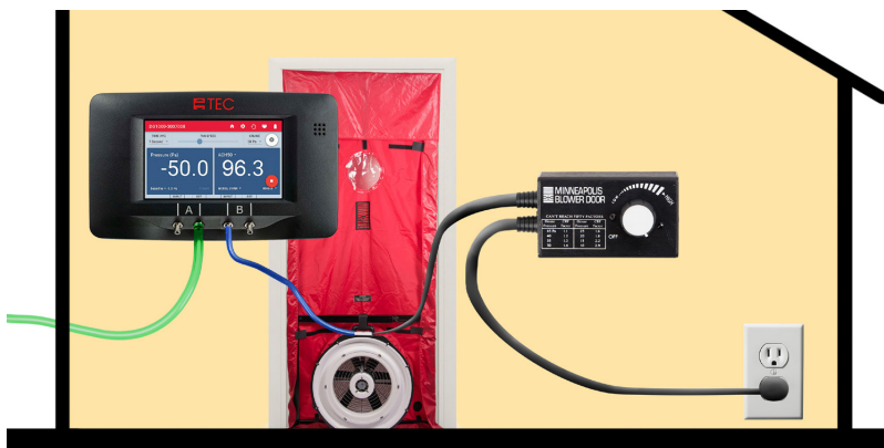
Figure 4. How blower door components are connected.
