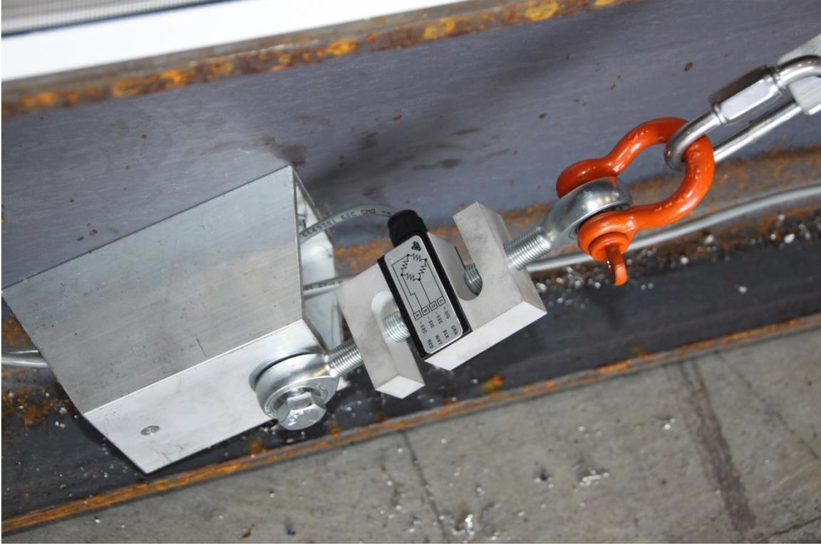
Figure 8. Load cell measuring the cable tension
