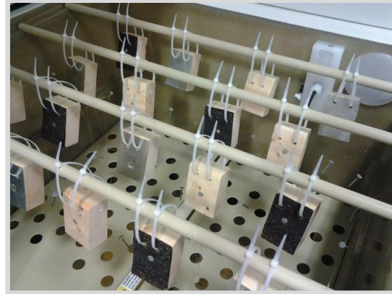
Figure 1: Images of the prepared roof fastener specimens within the test chamber
