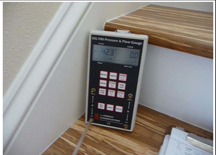
House significantly depressurized w/ kitchen exhaust.
