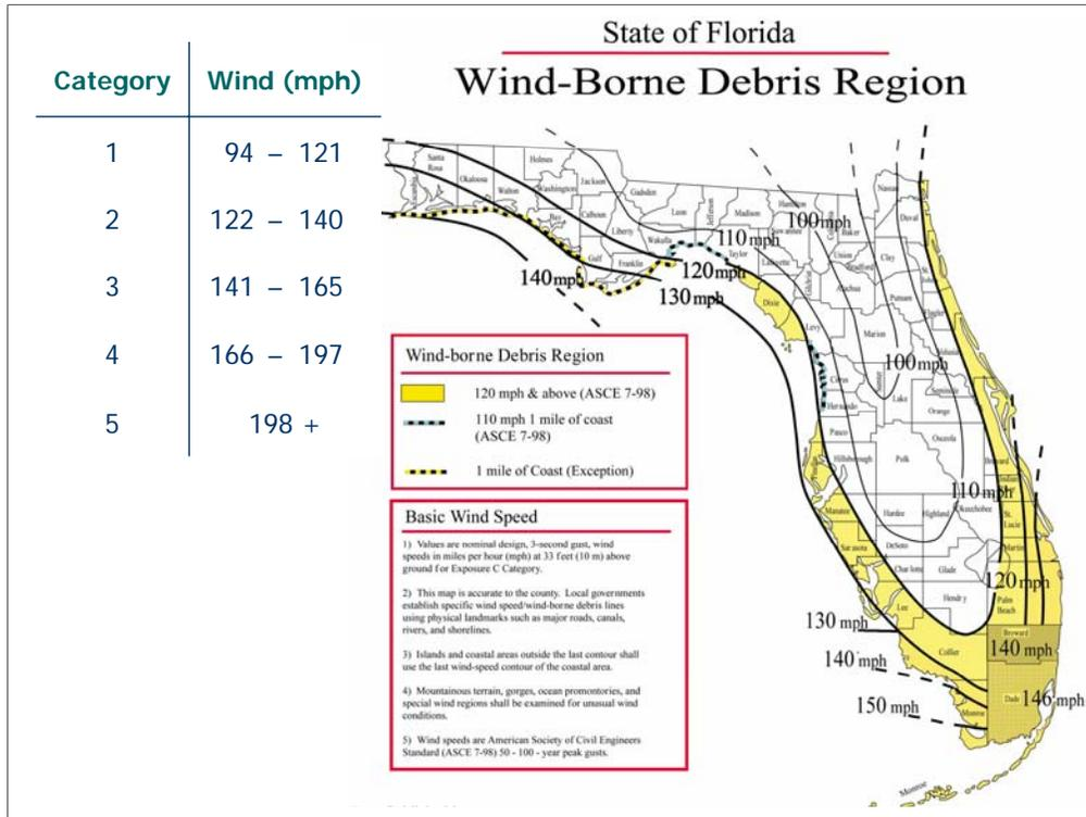
Figure 1609 *State of Florida Wind-borne Debris Region and Basic Wind Speed* map. The Florida map indicates the basic design wind speeds and the wind borne debris regions and is accurate to the county.
