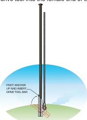
Hold the threaded rod and the drive tool together in one hand and use the sledge to hammer the drive tool, threaded rod and anchor into the ground.
