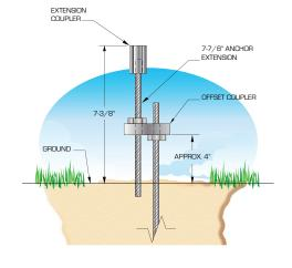
Turn the first MESA upside down and attach the four soil support pads (32 x 3" L shapes) by pressing them into the slots. Place the MESA unit into position, centering the coupler end of the anchor extension over the center hole. Check to make sure it is sitting flat and level.
