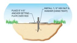
With the deep wall socket and 3/8" drill, tighten down on the hex nut. As the threaded rod is drawn up the anchor will set itself to the anchored position. There must be 4" to 6" of threaded rod above ground when the anchor is set. Remove the nut and anchor setting plate and keep for the next installation.
