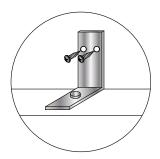
15 The hole in the side of each MESA is for the building inspector to view your anchor installation. The cover plate snaps into the hole and should be left loose until the installation is inspected. You or the home owner can easily attach them afterward.
