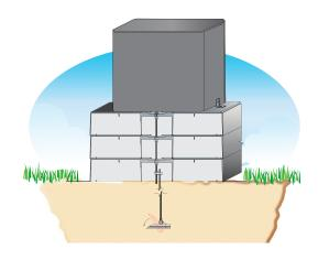
10 Attach the clips to the MESA first - use a 3/8" bit to drill through the hole in the clip and though the top of the MESA. With the clip placed over the hole, push an AVK fastener through the hole in the clip and through the hole in the MESA. The fastener sits on top of the clip - not under it.
