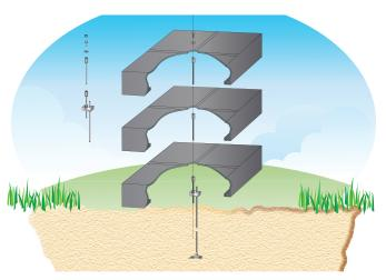
Using care, place the condensing unit on top of the MESA. Do not drop! The raised areas on the top surface of the MESA will indicate the best position for the unit and fastening clips. Determine the correct condenser position and all 4 clip locations before you drill.
