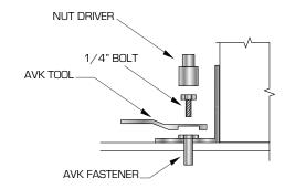
11 Place the fastener tool over the fastener flange and thread a 1/4" x 20 x 1-1/4" S.S. bolt through the hole in the tool and into the fastener a few turns to get it started. Use a variable speed drill with a 7/16" nut driver - apply some downward pressure and turn the bolt until it pulls the fastener tight. The fastener tool helps to keep the fastener from spinning out. Remove the bolt to release the fastener tool.
