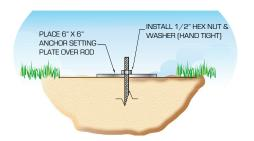
With the deep wall socket and 3/8" drill, tighten down on the hex nut. As the threaded rod is drawn up the anchor will set itself to the anchored position. There must be 4" to 6" of threaded rod above ground when the anchor is set. Remove the nut and anchor setting plate and keep for the next installation.
